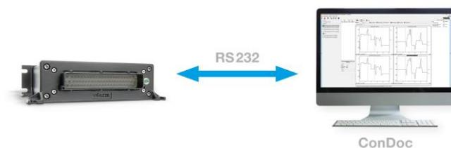
ConDoc is a terminal program which reads the data directly from the controllers and displays them in an ordered data structure. Each controller is equipped with standard values which serve as a basis for the individual settings.
